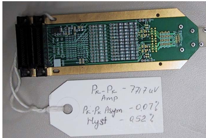
Figure 6-2 – BlazerX6 Hall Effect Probe Card
