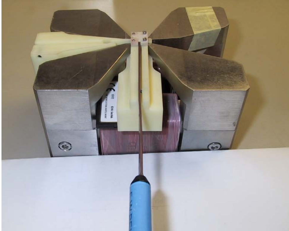
Figure 5-1 – BlazerX6 Quad-Pole Magnet Calibration
