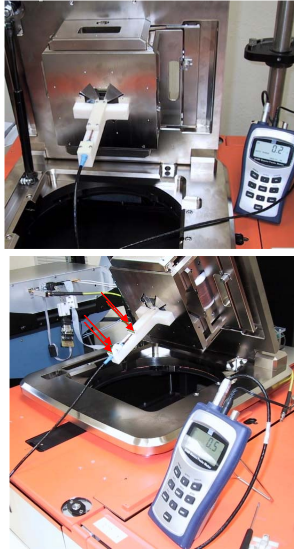
Figure 5-3 – WLA Quad-Pole Magnet Calibration
